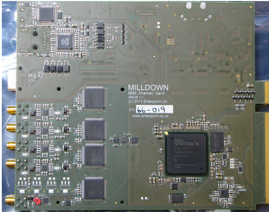
Figure 3.11: Front view of the Milldown DDS board. The 4 medium-size chips on the left are the integrated AD9910 synthesizers. The large chip on the right is the Spartan-6 FPGA. The top 4 SMA connectors on the left are DDS output ports, while the bottom connector is used as reference input. The region on the top-left is the internet-control unit, which we will not use in this experiment.
