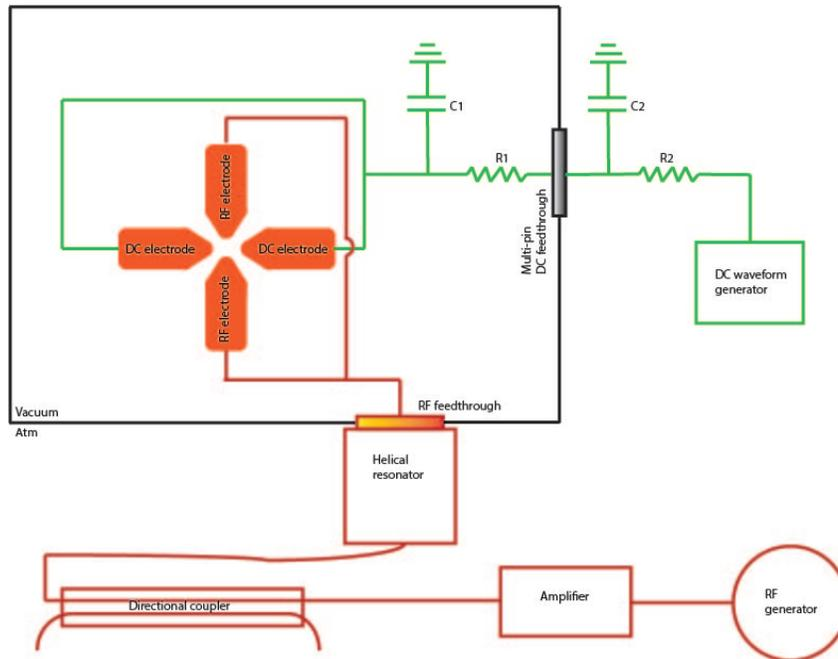
Figure 3.2: A schematic of the DC and RF power supplies of the system and how they are wired to the trap electrodes.
