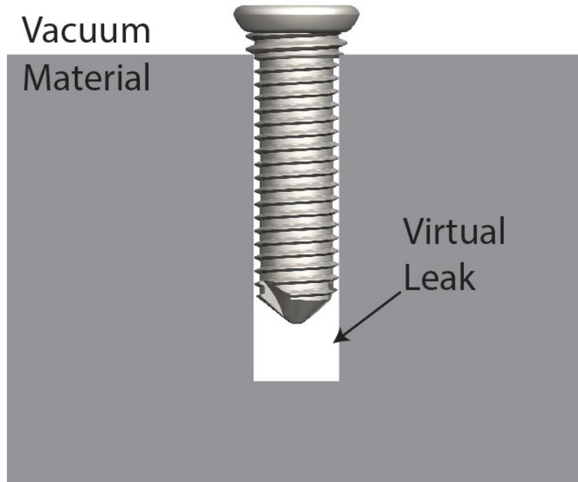
Figure 3.4: An example of virtual leak due to air trapped inside a cavity enclosed in a threaded hole.
