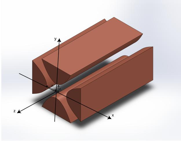
(a) Rod electrodes. Endcap electrodes are not shown in this diagram for clarity.
