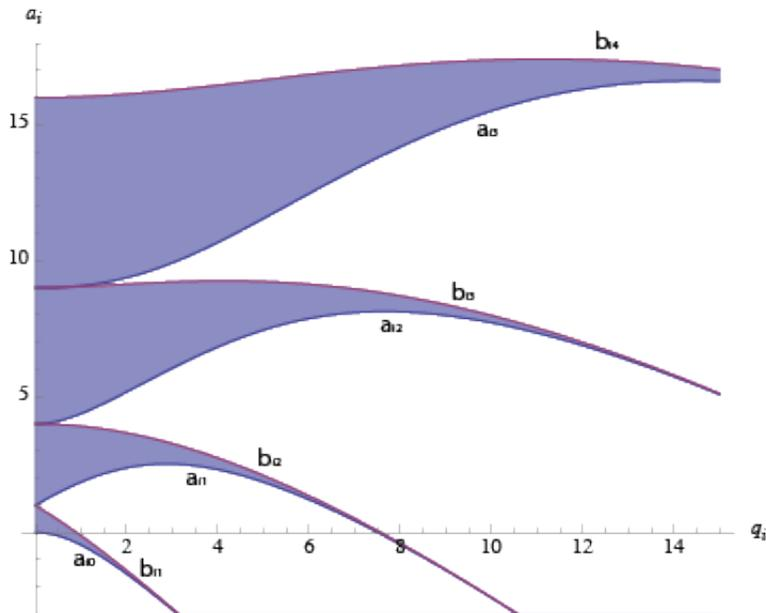
Figure 2.2: Stability regions (shaded) in an arbitrary dimension. The boundaries of these regions are functions of  $a_i$  in terms  $q_i$ . Setting  $\beta_i$  to 0 gives  $a_{i,2n}$  and  $b_{i,2n+2}$  while setting  $\beta_i$  to 1 gives  $a_{i,2n+1}$  and  $b_{i,2n+1}$ .
