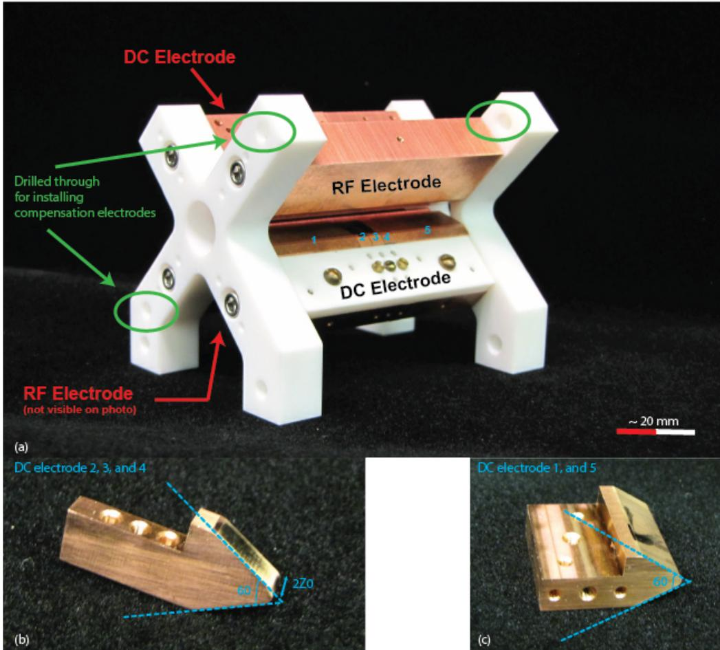
Figure 2.5: The assembly of electrodes of the actual linear Paul trap we have machined.
