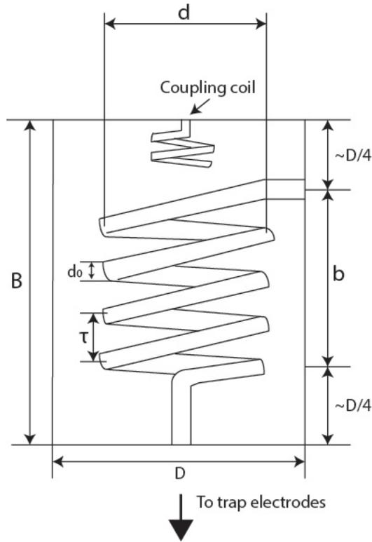
Figure 3.3: A schematic diagram of the helical resonator. The resonator coils and shield are made of copper. The shield is grounded.
