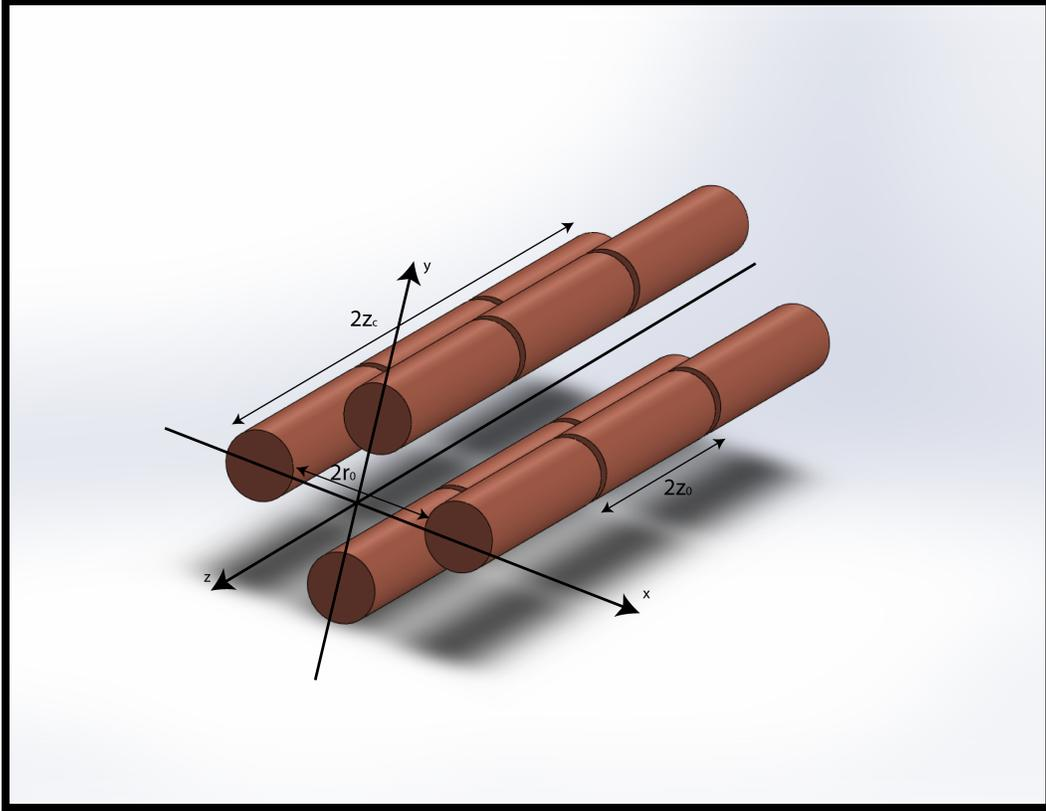
Figure 2.6: Cartoon of a real trap that consists of four thin linear segmented conductors set parallel and equally spaced around the  $z$ -axis, and at equal distance  $r_0$  from it. The endcap electrodes in this case are the four outer segments where the DC potential  $U_0$  is applied. The RF potential is applied to the inner segments.
