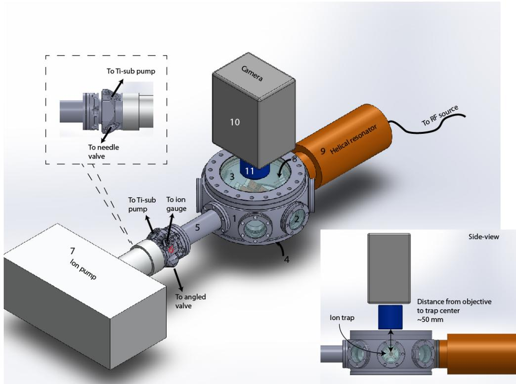
Figure 3.1: A schematic of the Paul trap system, including the main vacuum chamber, power supplies for the trap electrodes, the UHV pumping system and the imaging system.
