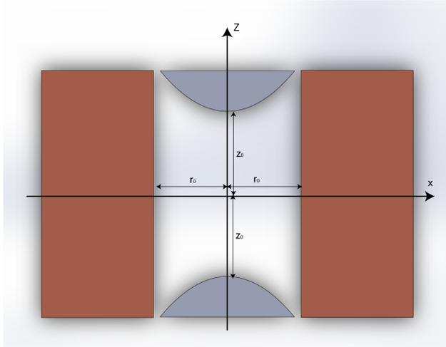
(b) Endcap electrodes, seen as a cross-section in the  $xz$ -plane. They are colored grey.
