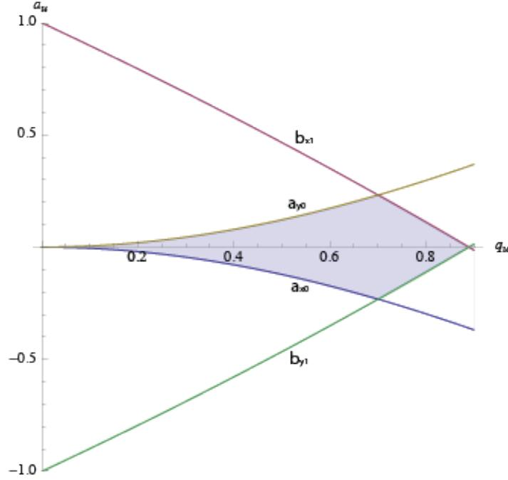
Figure 2.3: The stability region of interest for confinement in both x- and y-dimensions
