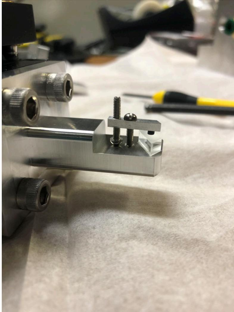
Figure A.5: BBO sitting in the custom mount, machined by Jim Kubasek. A small pocket was cut for the crystal to rest in, and the two-screw clamp holds it in place. The mount attaches directly to a stock Newport 9081 5-Axis aligner. A small piece of O-ring was placed between crystal and metal clamp to reduce mechanical stress on the crystal, which could induce unwanted birefringence.
