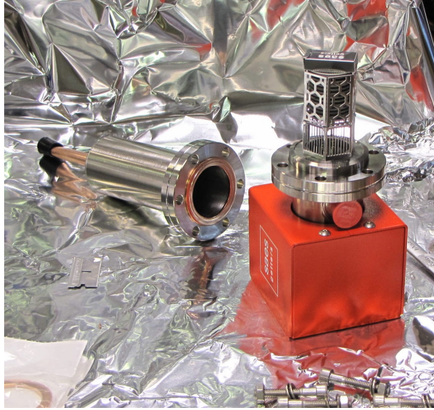
Figure 2.6: Getter and ion pump used for the vacuum chamber with the getter surfaces exposed. The getter materials are the disks within the hexagonal cage, while the ion pump is located out of view inside the red box. The dimensions of the red box are 6.5 cm x 7.5 cm x 8.5 cm.
