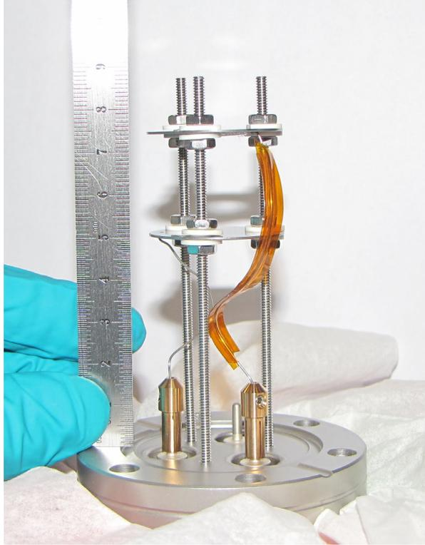
Figure 4.12: Photograph of the final electrode assembly. A side view of the assembly is shown, in which you can see the mounting washers and bolts holding the electrodes in place. In addition, the bare wire from the bottom electrode, and the Kapton-taped wire from the top electrode, are visible. The major markings on the ruler to the left are in cm.
