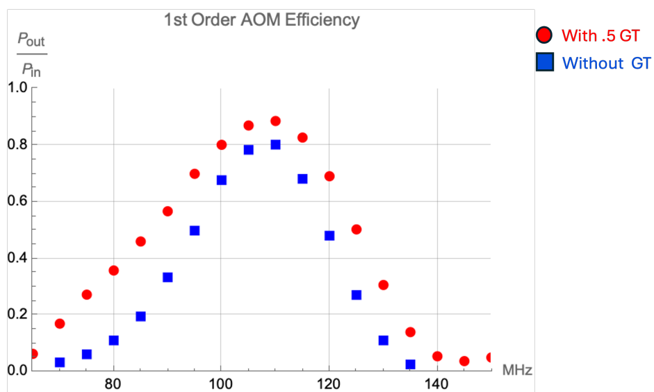
Figure 3.13: The AA Opto-electronics MT110-B50A1.50-IR AOM's first order efficiency with (in red) and without (in blue) the Galilean telescope of magnification .5. When using the Galilean telescope, we get better efficiency at every driving frequency.
