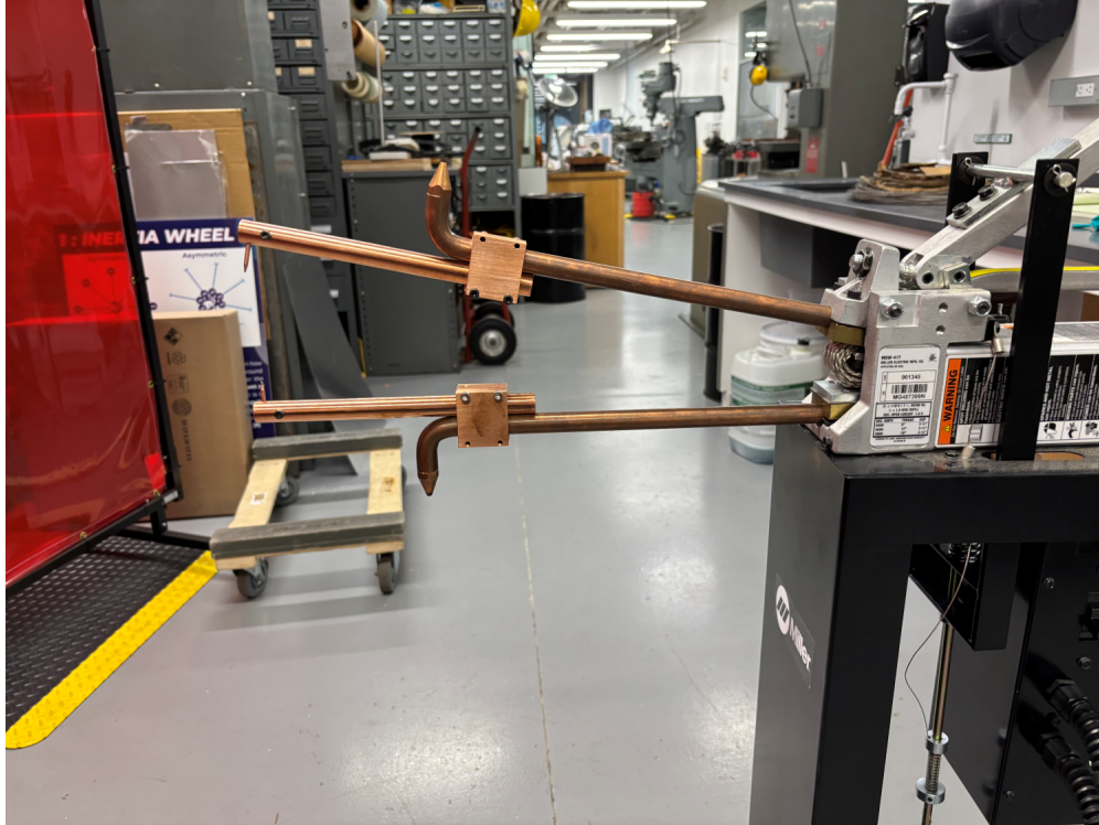
Figure A.2: The Miller Electric MSW-41T spot welder, with 12-inch copper electrodes, additional 6-inch extension, and Amada Tech ES0813 tungsten electrode tips.
