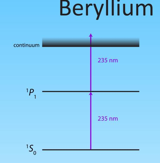
Photoionization laser: • Commercial diode laser (470 nm, 100 mW) • Second-harmonic generation in BBO Monolithic cavity design Similar to S. Hannig, *et al. RSI* **89** 013106 (2018) • Digital servo for lock
