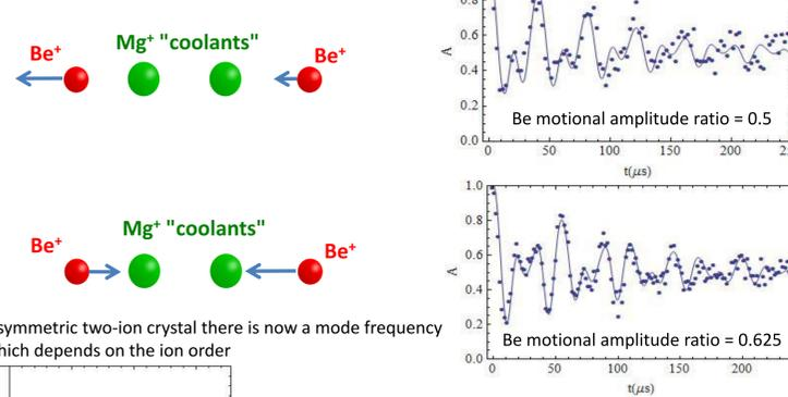
In an asymmetric two-ion crystal there is now a mode frequency shift which depends on the ion order
