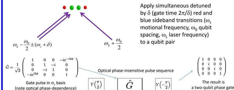
Apply simultaneous detuned by  $\delta$  (gate time  $2\pi/\delta$ ) red and blue sideband transitions ( $\omega_z$  motional frequency,  $\omega_0$  qubit spacing,  $\omega_L$  laser frequency) to a qubit pair
