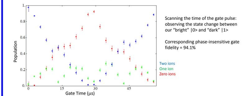
Scanning the time of the gate pulse: observing the state change between our "bright"  $|0\rangle$  and "dark"  $|1\rangle$
