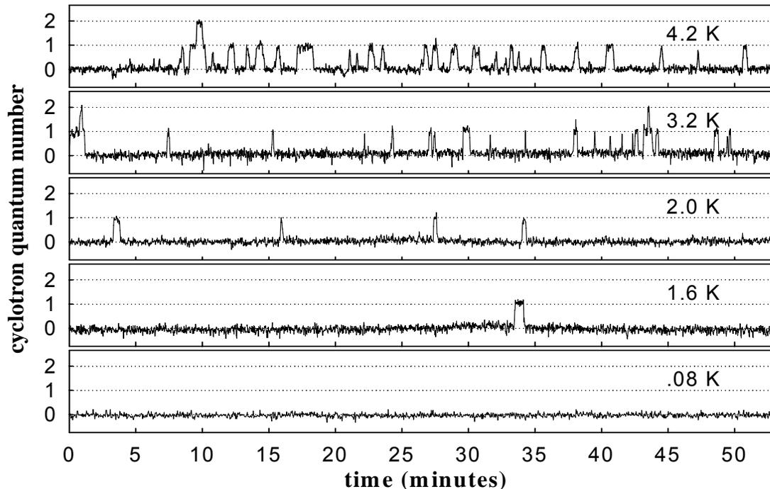
Thermal jumps are eliminated as the trap temperature is decreased from 4.2 K to 80 mK.
