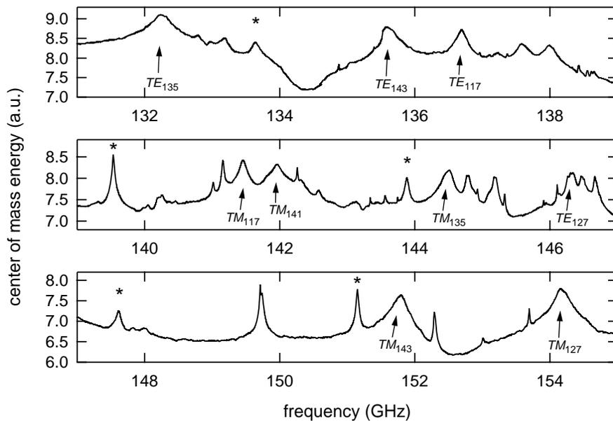
Measuring the cyclotron frequency on several features (\*) allows us to calibrate our mode maps.
