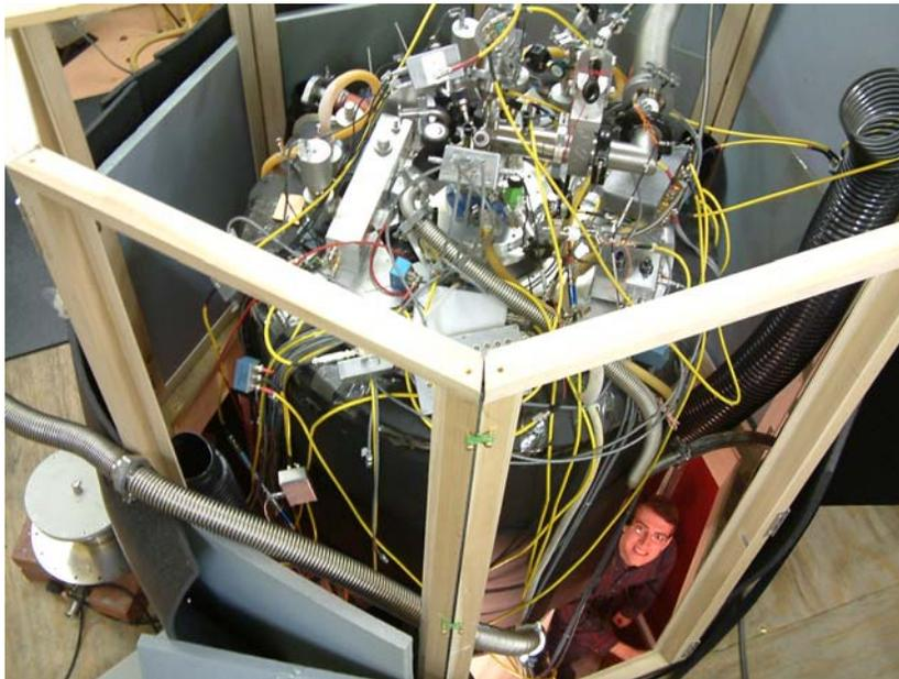
A 5.3 T superconducting magnet provides the field for the Penning trap. A dilution refrigerator keeps the trap electrodes at 100 mK.
