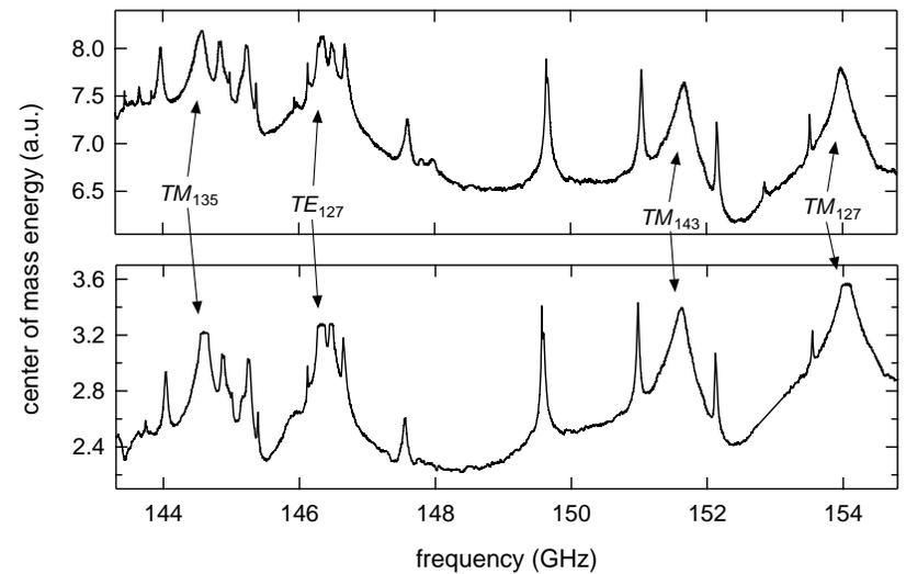
Strongly-coupled modes saturate as the number of electrons is decreased from  $3 \times 10^4$  to  $1.6 \times 10^4$ .
