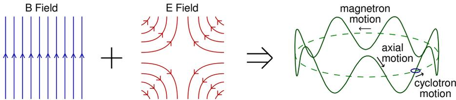
A uniform magnetic field confines the electron radially, while a static quadrupole electric field confines it axially. The slow magnetron motion is caused by the electron's  $\mathbf{E} \times \mathbf{B}$  drift.
